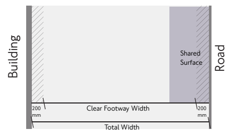
Loading Bays- shared surface
